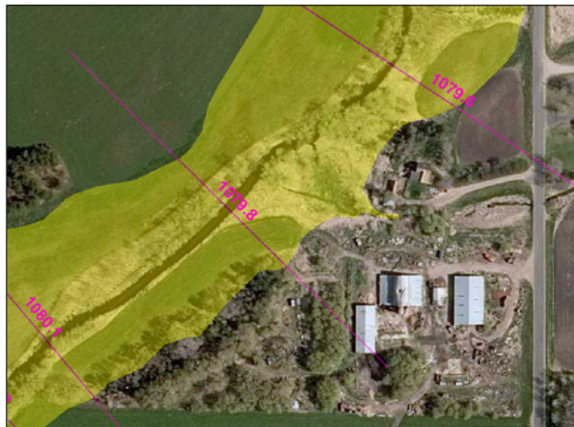
Sample showing “pink lines,” which are estimated 1% Water Surface Elevations that can be used as best available data BFEs.
